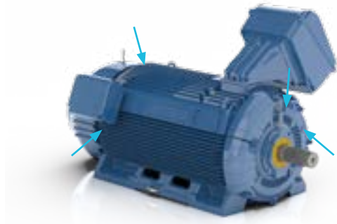
Figure 39 - Location of vibration measuring points.
