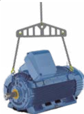
Figure 8 - Lifting with inclined chains.
