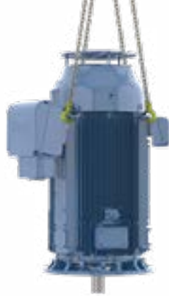
Figure 9 - Lifting of vertical motors.
